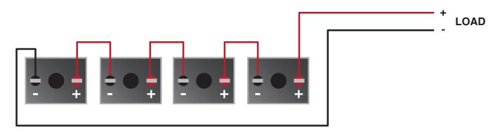
Note: When using LiFePO4 batteries in circuits, NEVER mix brands, capacities or voltages. Always use identical batteries in your circuit (ie: same brand/model, same amp hour (Ah) rating, same voltage).
